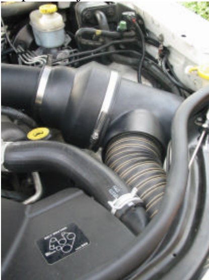
Step 7 – Slide hose onto inlet. Make sure hose is not pushing canister, if it is, push hose further into grill opening and / or trim small amounts of hose until it fits.
