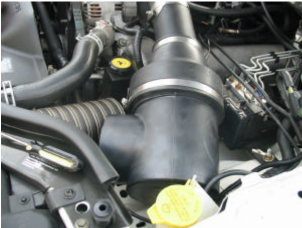
Step 6 – Adjust canister so filter is centered, and hose inlet is in position, tighten clamps
