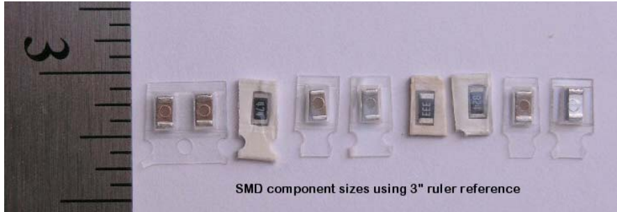
SMD component sizes using 3" ruler reference
