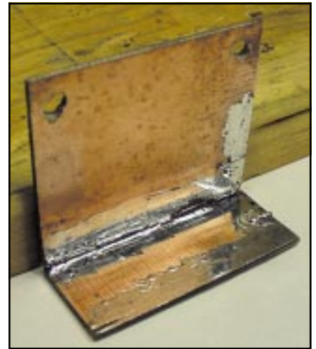
Figure 7—Use a poor ham's 90° jig when soldering the boards.
