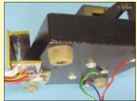
Figure B—The keyer mounted on a Kent Paddle. Build the circuit on a U-shaped set of boards to fit your paddle. The circuit board and battery board will fit under the paddle and only the pushbuttons and piezo buzzer will be visible on top.
