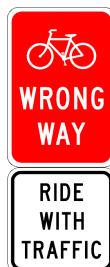
Bicycle Wrong Way (R5-1b) and Ride With Traffic (R9-3c) signs (Section 9B.06)
