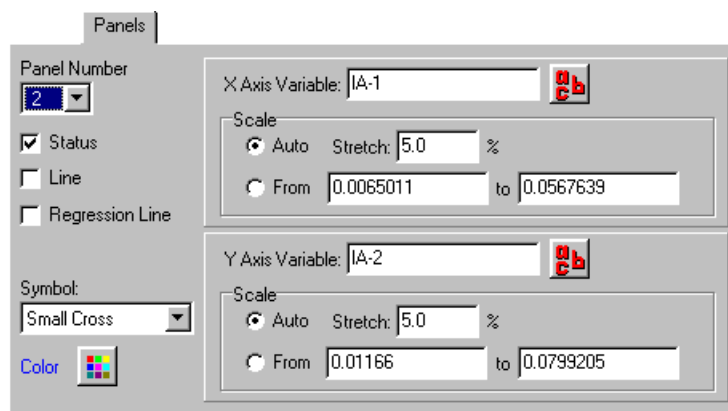
Figure H-25. An example of the Panels tab of the format parameters window associated with the graphical range filter display.
