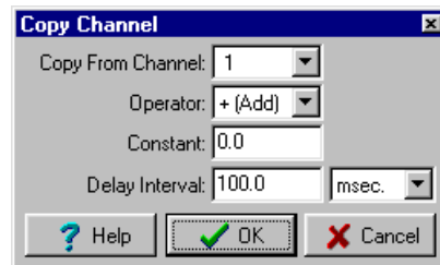
Figure D-3. The parameter window associated with the Copy Channel processing option.
