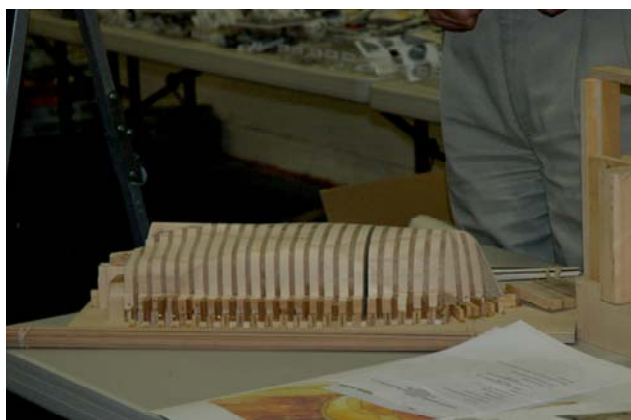
Side view of framing "jig"
