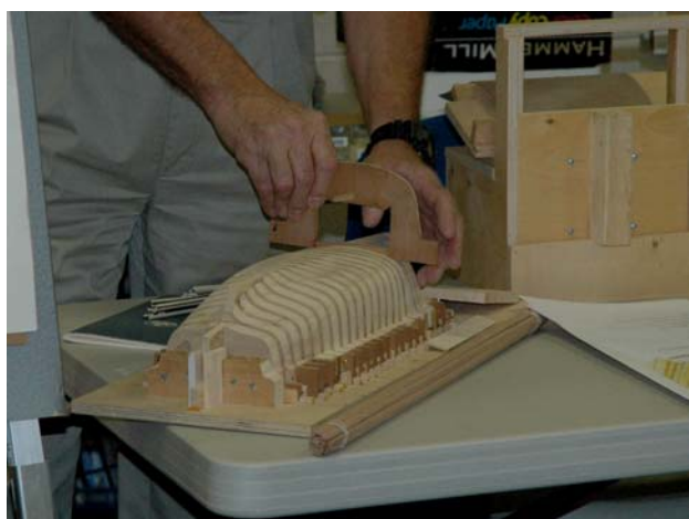
Inserting shaped frame into jig
